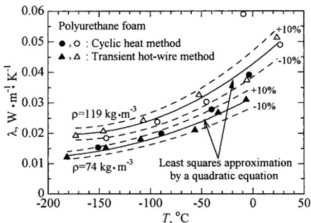
**Fig. 3.** Thermal conductivity  $\lambda$  of polyurethane foam with a bulk density  $\rho=74$  and  $119 \text{ kg}\cdot\text{m}^{-3}$ . ●, ○ measured by the cyclic heat method; ▲, △ measured by the transient hot-wire method; least squares fit of the measured results; ---  $\pm 10\%$  deviations from solid line.
