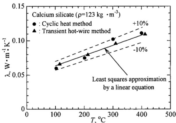
**Fig. 4.** Thermal conductivity  $\lambda$  of calcium silicate with a bulk density  $\rho=123 \text{ kg}\cdot\text{m}^{-3}$ . ● measured by the cyclic heat method; ▲ measured by the transient hot-wire method; — least squares fit of the measured results; ---  $\pm 10\%$  deviations from solid line.
