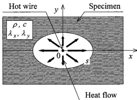
Fig. 1. Physical model and coordinate system of anisotropic material.
