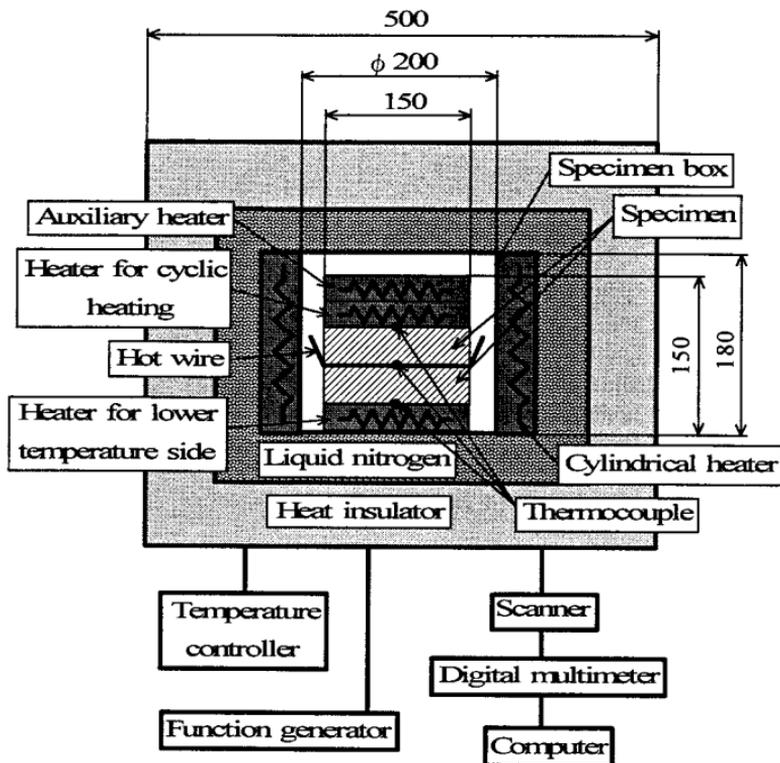
Fig. 2. Schematic of apparatus for thermal conductivity measurement of thermal insulations. All dimensions are given in mm.
