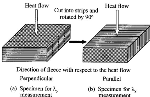
**Fig. 7.** Schematic of fibrous insulation.
